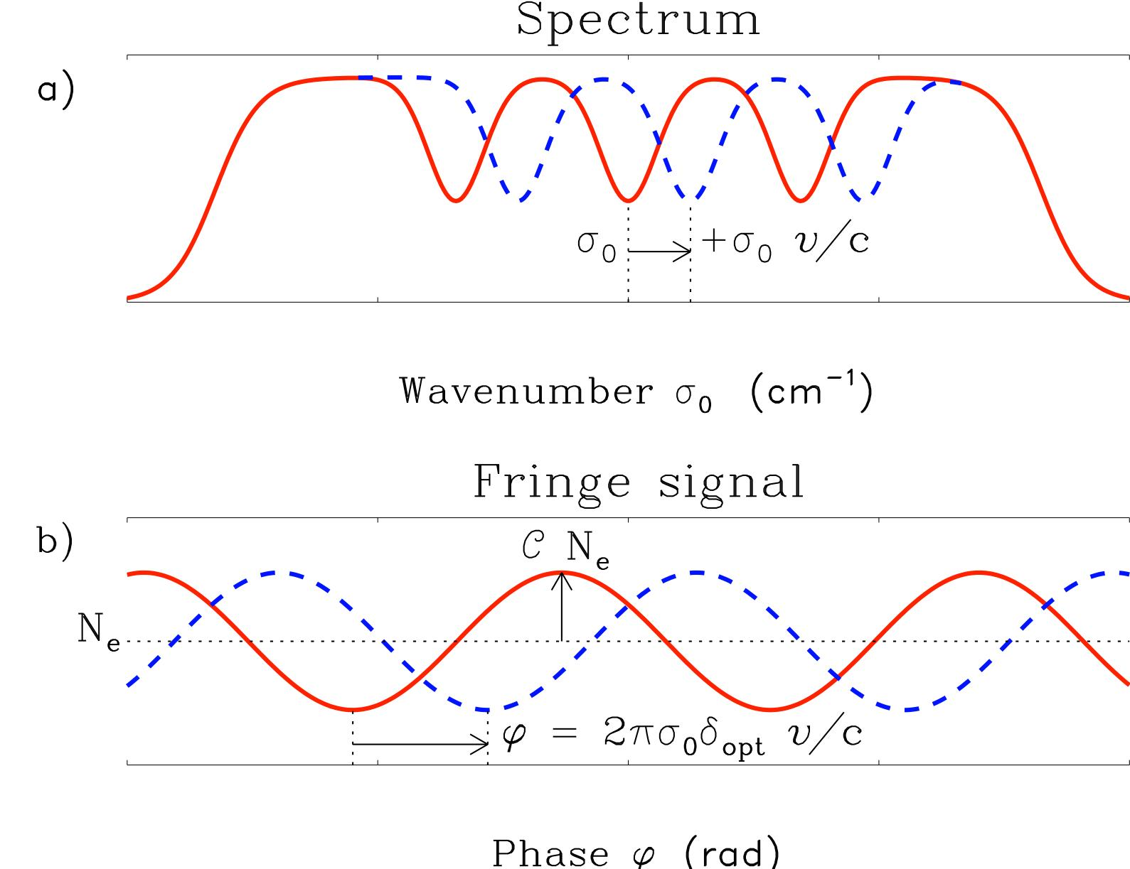
The repeated recording of the same fringe allows us to construct the Doppler signal, related to the phase shift  $\varphi$  :
