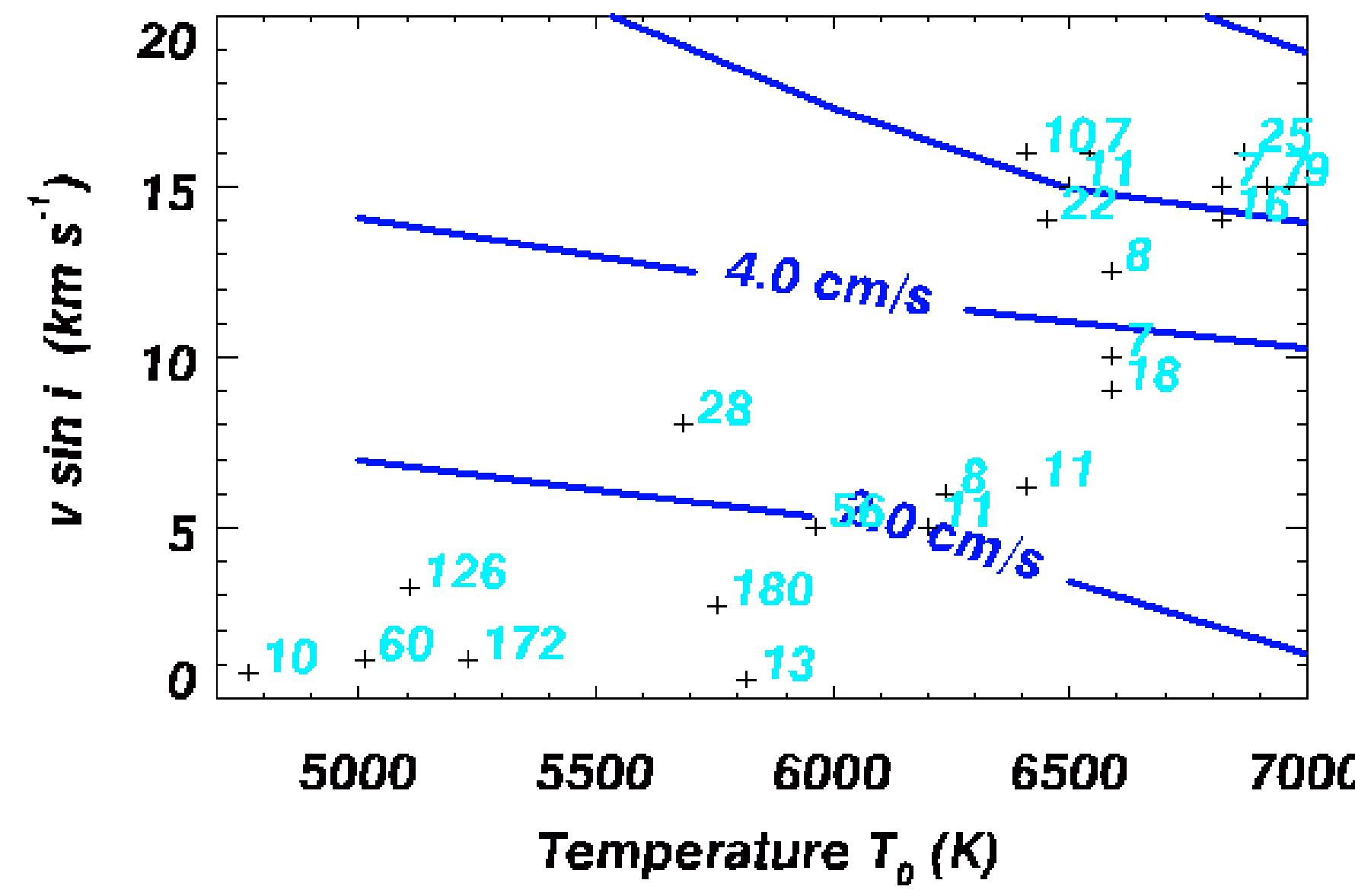
Isovelocity levels give the performance  $v_{rms}$  as a function of effective temperature and  $v \sin i$ , obtained in the following conditions : 2-m class telescope, 5 nights with a global duty cycle 95%, and 4th magnitude star.
